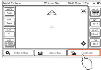
**Step 2)** Tap the 'Model Select' button, and if required press 'OK' to bypass any pop up warnings/alerts.
