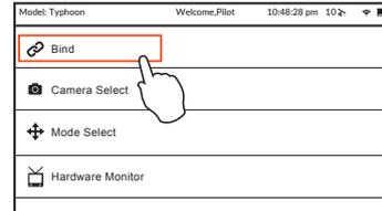
**Step 6)** Tap the 'Bind' button and select the 'CGO3\_XXXXXX' camera listed in the column under 'Camera', then enter the password '1234567890' when prompted and tap 'OK' after the connection has been established.
