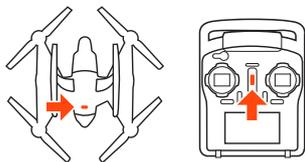
**Step 2)** Turn on the transmitter and allow it to boot up fully before turning on the aircraft. And when the transmitter and aircraft are powered on and linked proceed to the next step.
