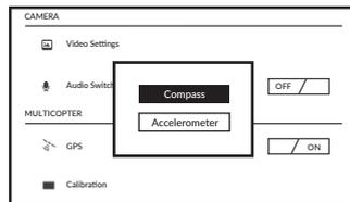
**Step 3)** Tap the Setting button on the ST10+ screen, then tap the Calibration button. Choose Compass option and tap it.
