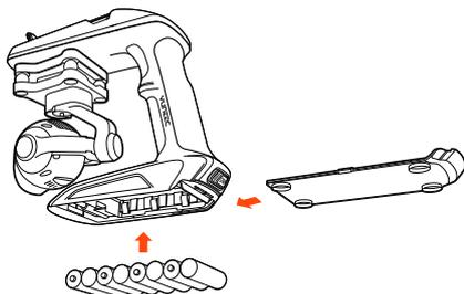
Slide the battery cover / door upward with slight force and inspect the AA battery compartment.
