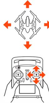
Angle (Pilot) Mode is the mode preferred by experienced RC/drone pilots because the TYPHOON will move in the direction the control stick is pushed relative to the front/nose of the aircraft. So if you push the right-hand stick to the left the TYPHOON will bank toward the left side and move to the left. This means if the front/nose of the TYPHOON is pointing away from you it will move to the left, but if the front/nose is pointing at you the TYPHOON will move to the right.
