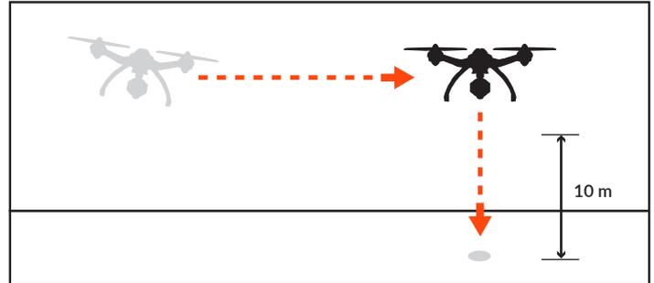
**B)** When flying lower than 33 feet (10 meters) the TYPHOON will climb to 33 feet (10 meters) while flying back to the home point, or active home position, then descend vertically until it lands.
