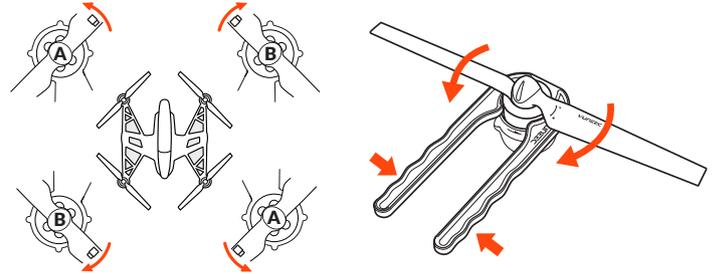
Each motor and propeller are marked with an 'A' or 'B' to ensure easy installation in the correct positions (for example: install propellers marked with 'A' on motors marked with 'A').
