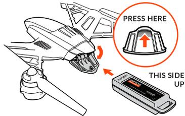
**STEP 1)** Push the area at the top of the battery door to release the latch/lock, and then open the door.
