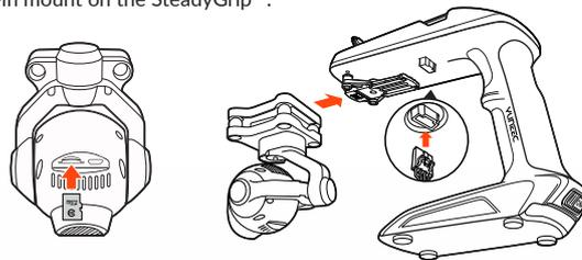
**STEP 2)** Carefully connect the CGO3's power/control connector to the power/control port of the CGO SteadyGrip™ and then insert a microSD card into the corresponding slot on the bottom of the CGO3. You can use the included 16GB card (from your RTF package) or any Class 10 microSD card up to 128GB.
