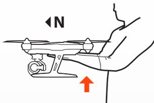
**Step 5)** When the main LED status indicator flashes red and green slowly (2 times per second) you have entered compass calibration mode. Pick up the aircraft and hold it flat with the nose pointed to the north. After 5 seconds the main LED status indicator should flash red and green rapidly (5 times per second).
