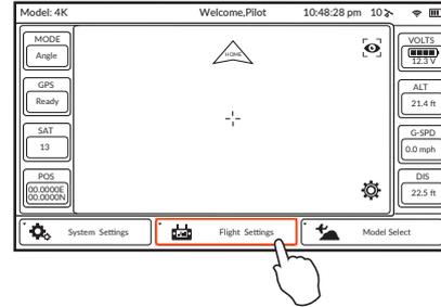
**Step 5)** Tap the 'Flight Settings' button, and if required press 'OK' to bypass any pop up warnings/alerts.
