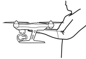
**Step 10)** The main LED status indicator should be flashing red and green rapidly (5 times per second). Hold the aircraft as still as possible until its main LED status indicator stops blinking rapidly.
